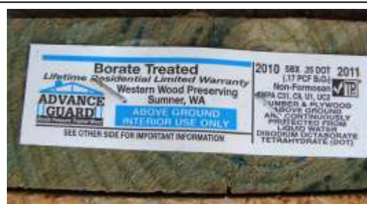
Figure 4-7 Borate treated lumber is not toxic to humans, and does not increase corrosion in fasteners like other chemicals.
